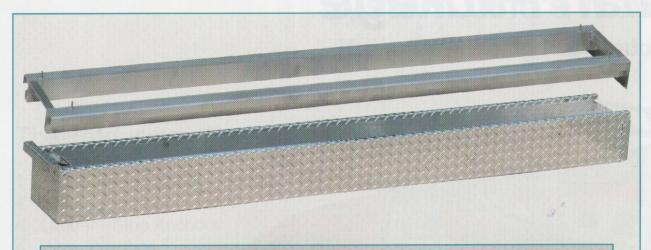
StowAway™ Drawers include the drawer, drawer slide rails and all stainless steel hardware to mount to the underside of top-side tool boxes. The drawer front hinges down for access to pullout trays or long items, or it can be secured in the closed position when used as a drawer. The locks can be supplied keyed alike to match our Full Access® Tool Boxes.
