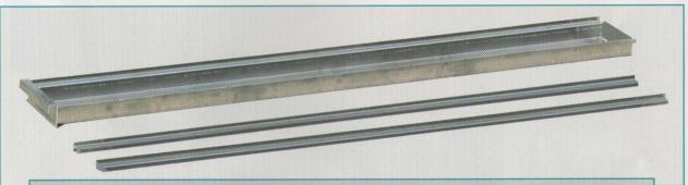
One or two Pullout Trays can be installed in StowAway™ Drawers. Sliding trays come with two sliding rails for each tray and are installed by drilling and mounting to the inside walls of the drawer. The drawer front is used in the "hinged position" Pullout Trays include the tray, tray slides and all stainless steel mounting hardware.
